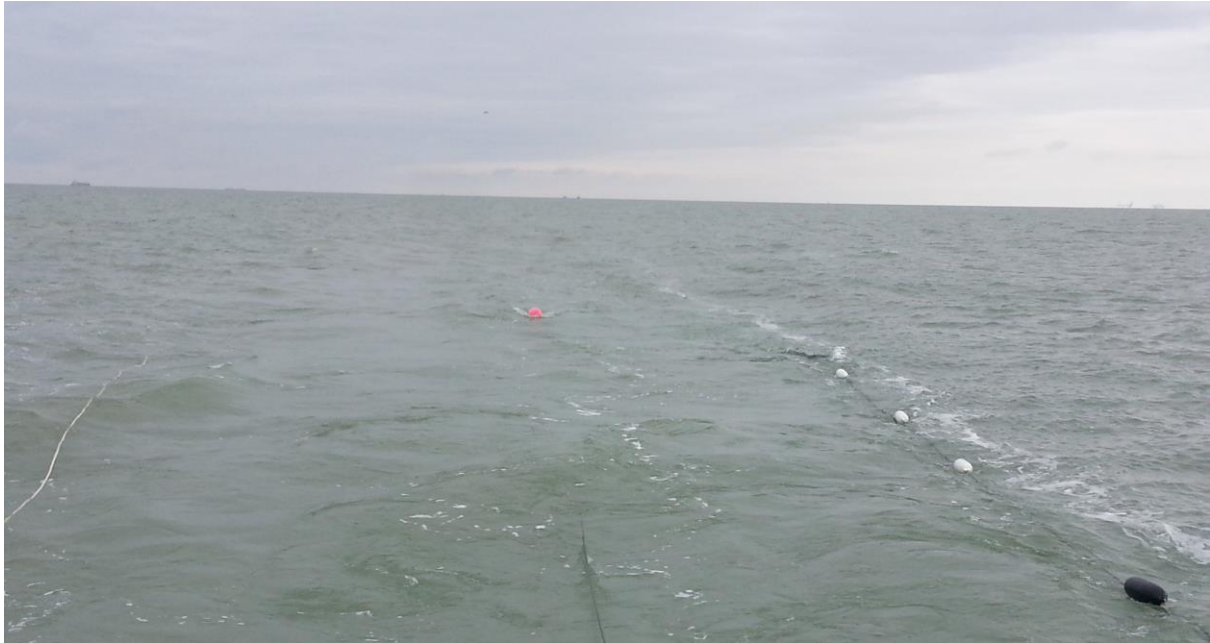
Figure 3: Data acquisition using two different streamers (SC = Single channel; MC = Multichannel, respectively left and middle) and a source (sparker or boomer; right side) towed behind the ship.
